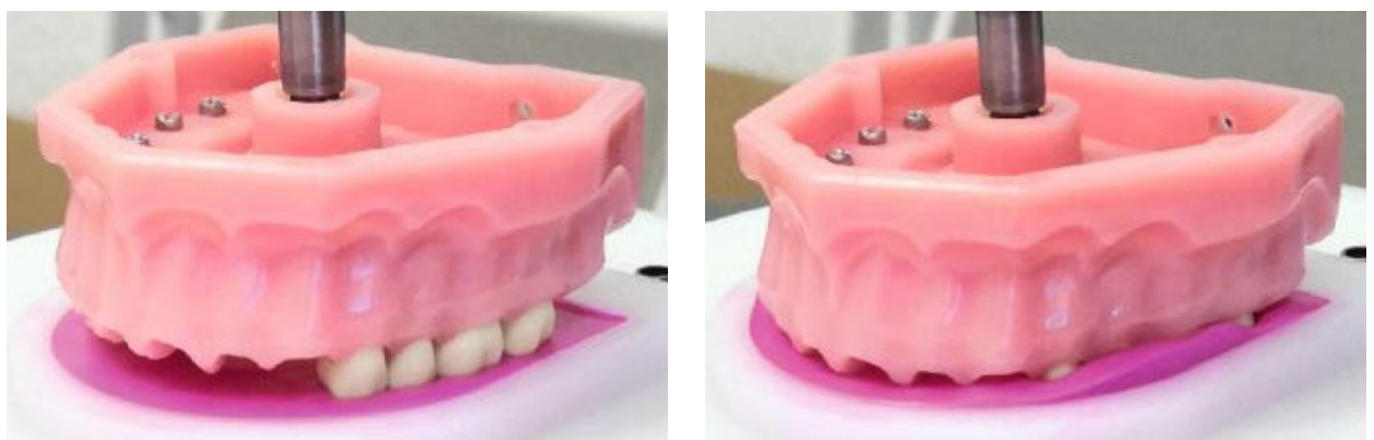
Fig. 6 Half of the difference in deformation force between 2x4 teeth and 2x2 teeth measured on the complete model should correspond approximately to the tilting force acting on the lower jaw when penetrating the registration material.
