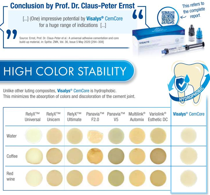
Light-cured samples, stored 48 h in the corresponding solution at 37 °C.
